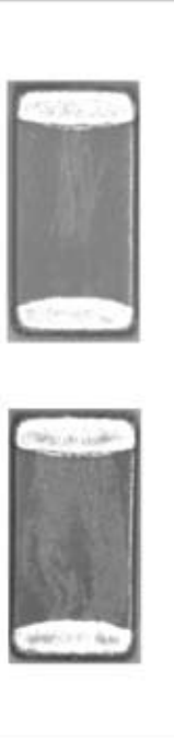
TYPICAL TERMINATION TO TERMINATION SURFACE ARCING ON MLCCS (shown in polarized light)
